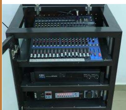
Top: Yamaha MG24XU Digital Mixer, Middle : QSC Speaker System & Bottom : Studiomaster SPS-8 Channel Power Sequencer
