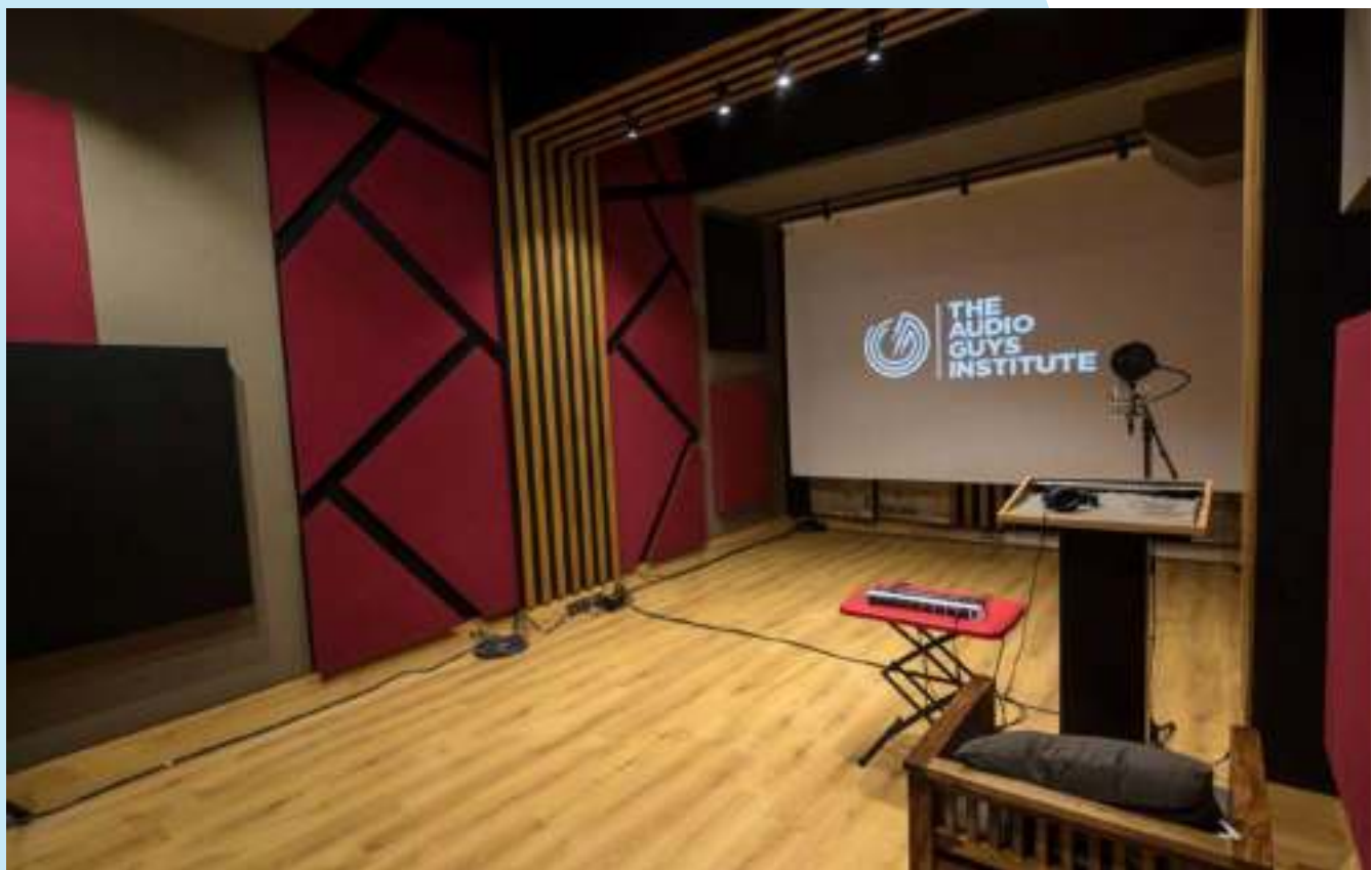
Studio C - Live Room features a live-end dead-end scheme with more absorption
